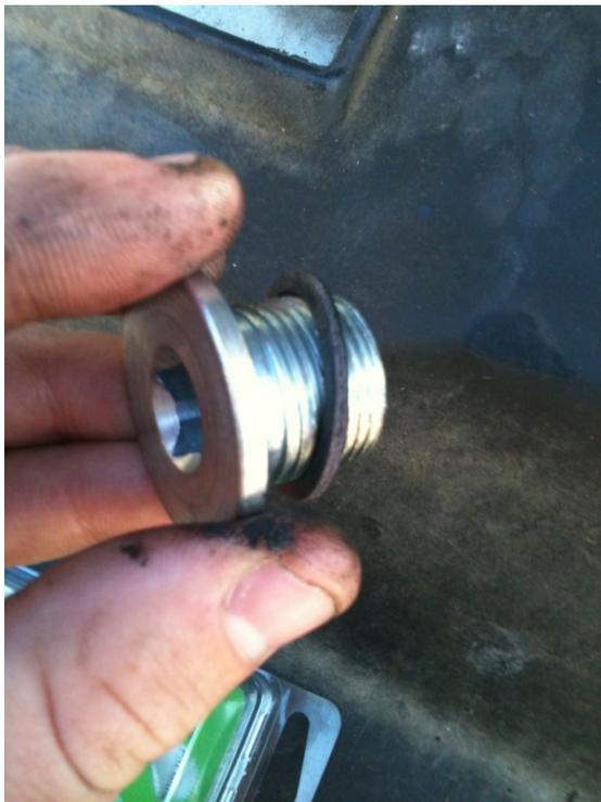
This plug will just screw right in. Do not over tighten or you may strip the threads out.
