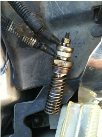
Additionally, you may want to wire in a resistor so no soft codes will be thrown if/when the AIH is supposed to be on. All you would have to do is run a 1 watt 470-ohm resistor from the post where the red wire originally went, then to a ground. A ½ watt 470-ohm resistor should work fine also(easier to find).
