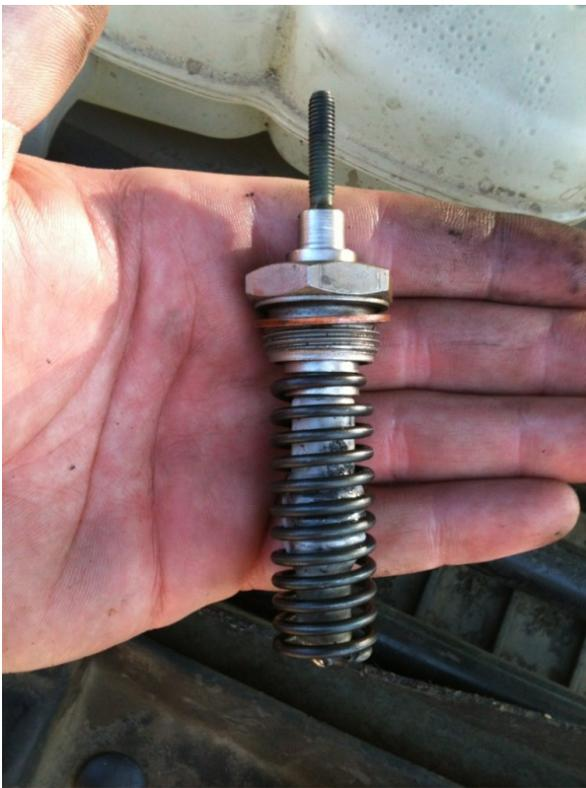
Now you must obtain a bolt to replace the AIH plug. It is a M22-1.5 bolt. You can get this new plug/bolt from some diesel product vendors or you can go to an auto parts store and get an oil drain plug for a 2000 Dodge diesel. I just used an oil drain plug.
