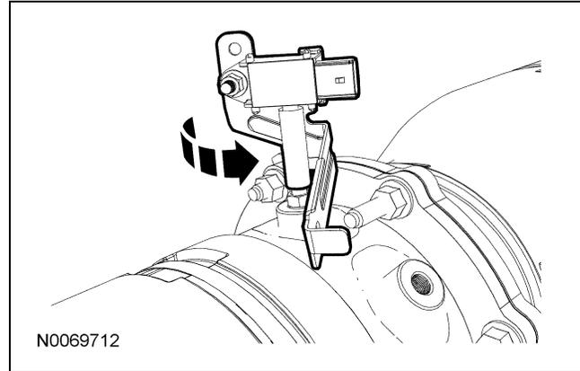
2. Install the diesel particulate filter pressure sensor bracket nut.
