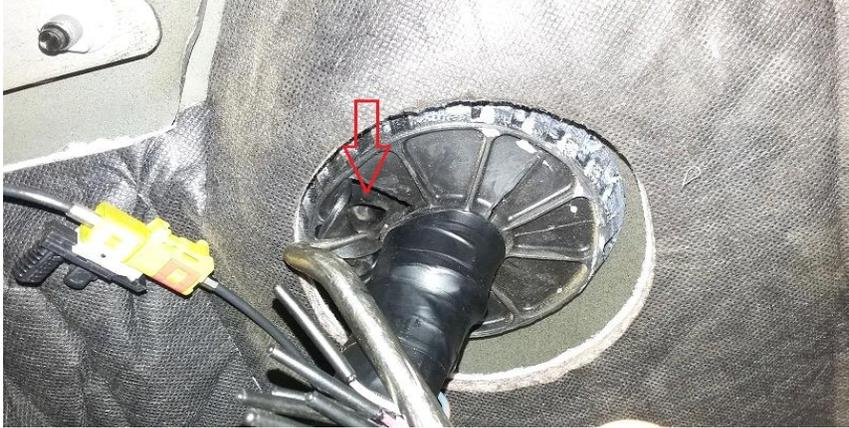
3. Locate the other side of the grommet in the engine compartment (next to the brake booster) and cut the tip of the protruding rubber cylinder.
