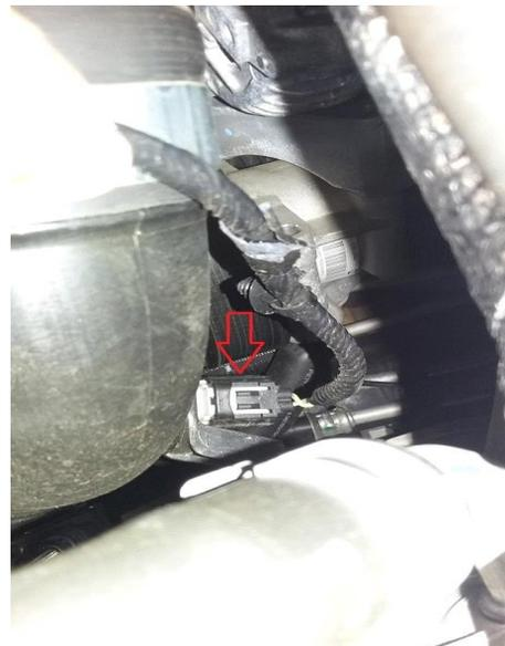
7. Reroute the charge air temperature sensor connector under the upper radiator hose and plug it into the SOTF cable adjacent to the battery (as depicted below). Route the SOTF cable between the battery and fender. Pull any excess slack in the SOTF cable from the engine compartment into the cab.
