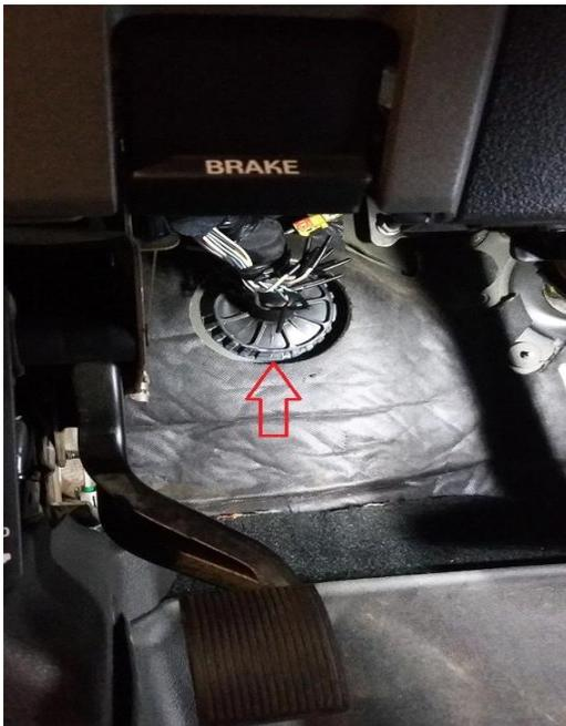
2. Make an incision in the grommet large enough to fit the SOTF cable through.
